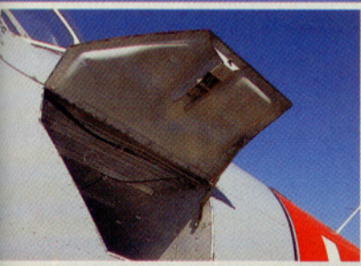
Initial reciprocation is announced by a generous dose of noise and lavish puffs of smoke (top). The modest baggage compartment behind the rear seat can hold 100 pounds of essentials (above).
