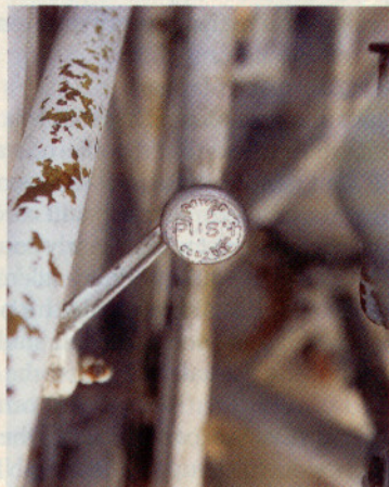
The austere monochromatic paint-schemed cockpit is open to the belly of the airplane with trays for the pilot's feet (above left). The left side of the cockpit is a busy place with rudder and elevator trim wheels, wobble pump handle, carb heat knob, gear handle, and flap lever (top right). The hydraulic power control lever activates the hydraulic system for about two minutes (above right).
